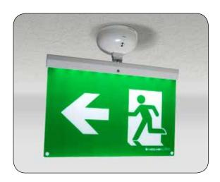
An LED-based, addressable 24m viewable exit light with a flexible 'flex it' hinge solution. The exit light's hinge cup contains the electronics and stand-by battery and allows the unit to attach to the Hochiki EL-TSB mounting base. The cup also features a bicoloured status LED indicating charge/fault status (green for charging, red for fault), approved to AS2293.
